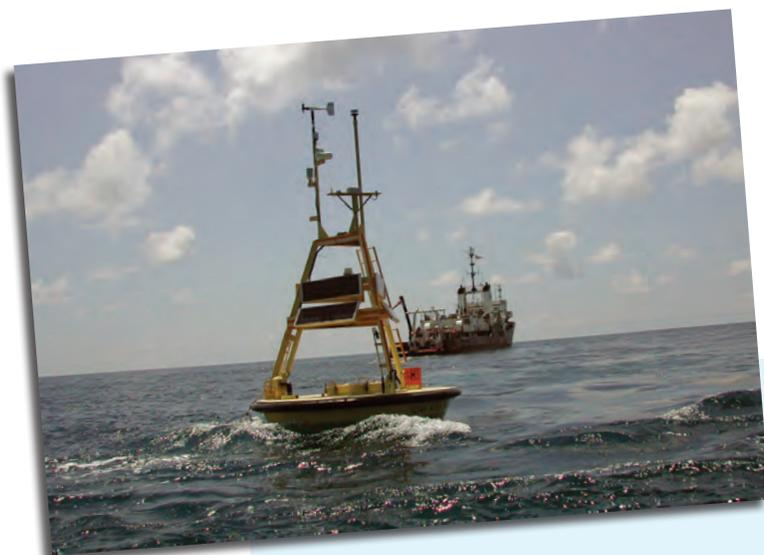
*One of the Texas Automated Buoy System (TABS) buoys, deployed to efficiently direct State and Federal emergency responders. The buoys also provide real-time oceanographic and meteorological data through GCOOS, the State of Texas, and the National Data Buoy Center. (Credit: Texas A&M University Geochemical and Environmental Research Group)*
